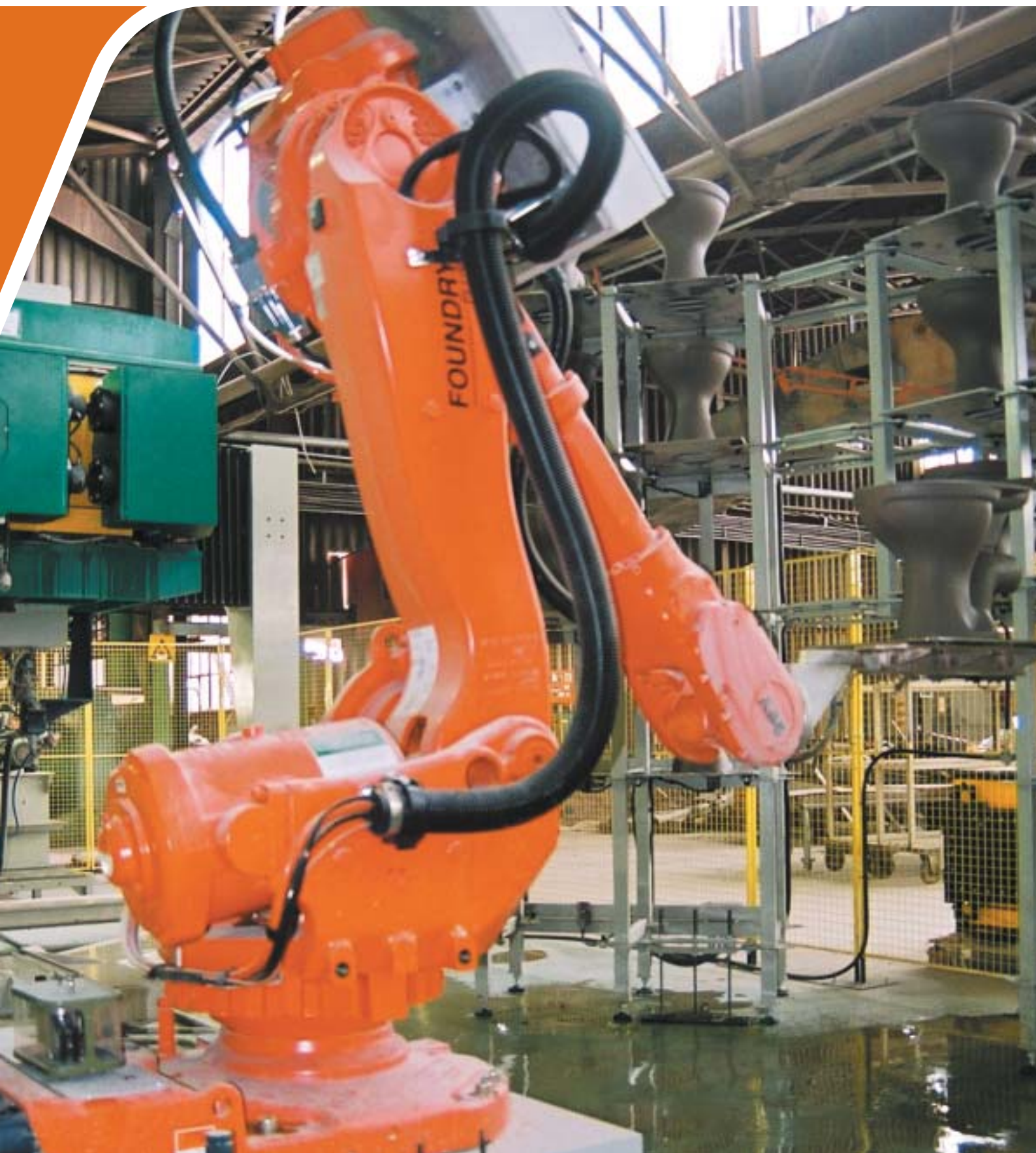
Vaal Sanitaryware - Robotic high-pressure casting technology
