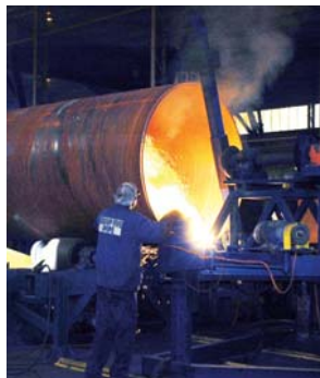
The manufacturing of spirally milled steel pipes takes place at the group's factory in Gauteng
