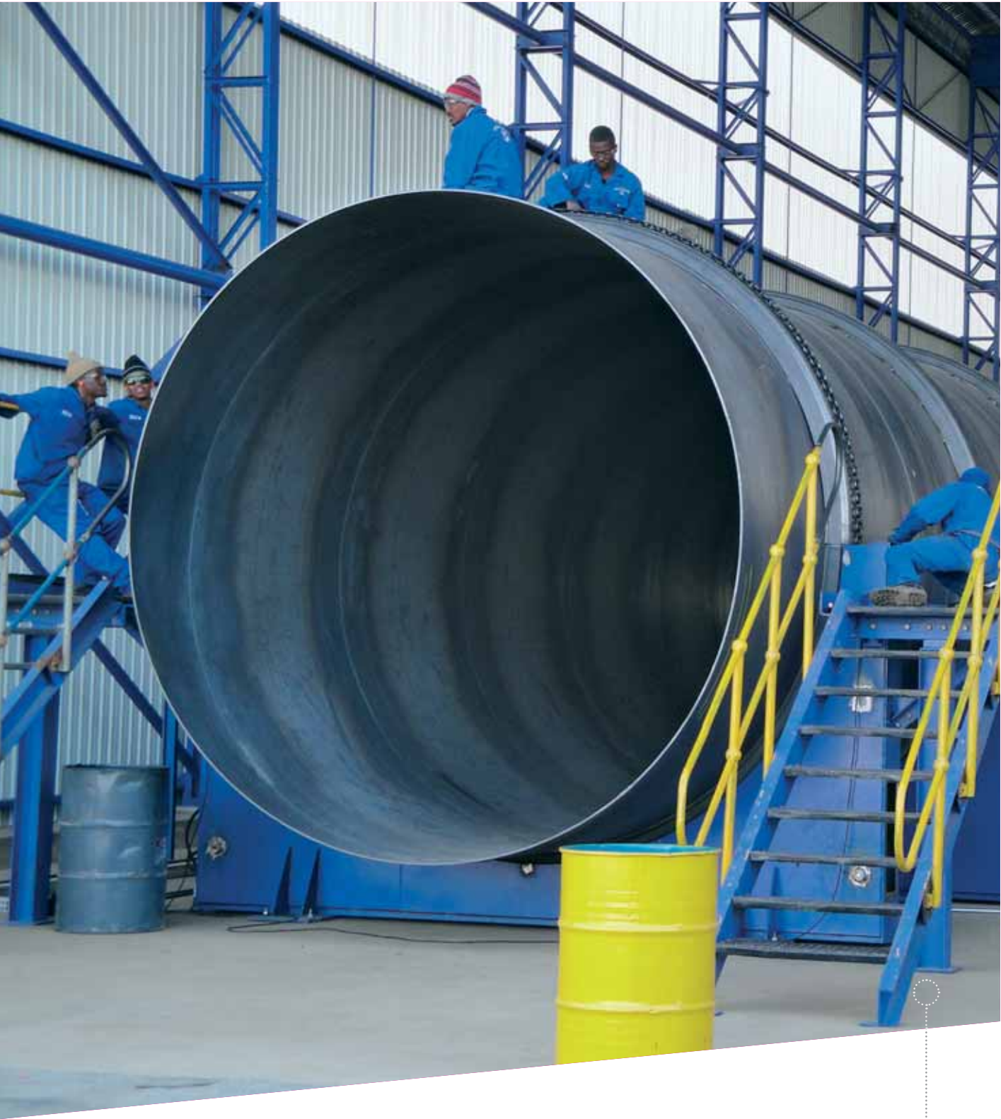
Large bore, spiral welded steel pipe, Group Five Pipe, Gauteng, South Africa
